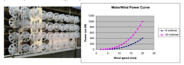
Figure 2.18: MotorWind turbine array and power curve
