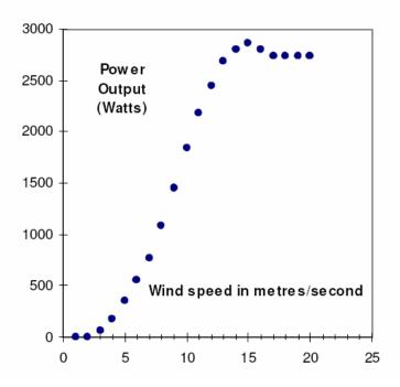
Figure 2.4: A typical power curve
