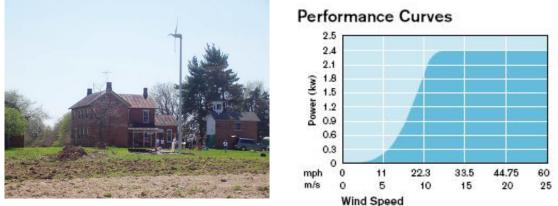
Figure 2.16: Skystream Turbine and power curve
