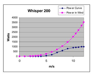
Figure 2.5: Whipser 200 Power Curve
